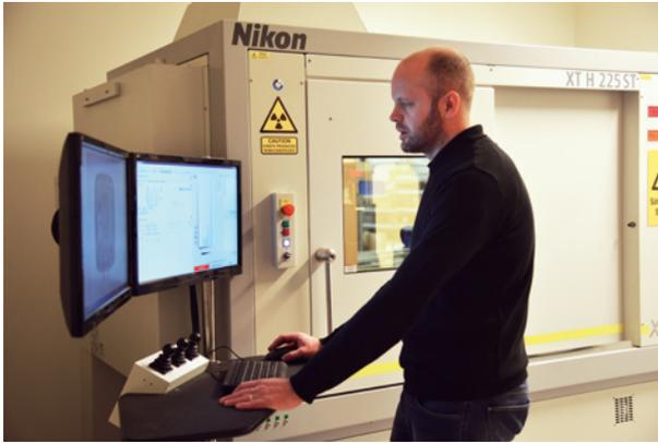
■ Carl-Anton Manns operates the Nikon Metrology XT H 225 ST, which is used to validate supplier samples and new parts at Nordic Lights.
