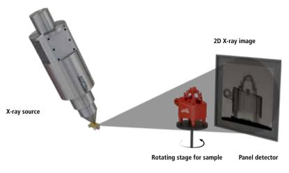
X-ray scans are taken at discrete positions of the rotating stage. Afterwards all slices are reconstructed to a 3D CT volume.
