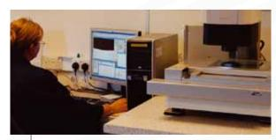
Monitoring manufacturing repeatability by checking pieces visually using the iNEXIV VMA-2520
