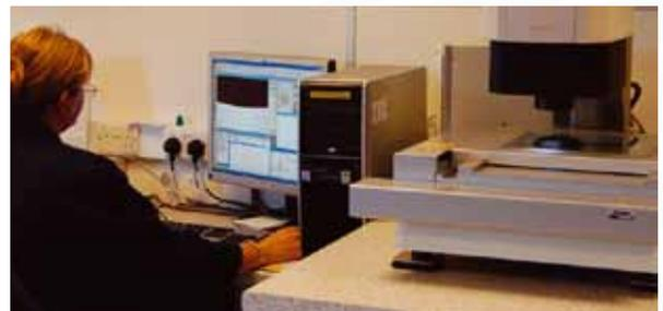
*Monitoring manufacturing repeatability by checking pieces visually using the iNEXIV VMA-2520*
